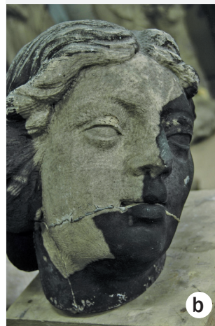
Fig.1.2.2. a) - Effect of deposition of soot, dust and pollutants on the look of busts that adorn the Czapski Palace - headquarters of the Academy of Fine Arts in Warsaw. b) - A head of a woman undergoing cleaning with pulsed laser radiation. Photo by A. Koss.
